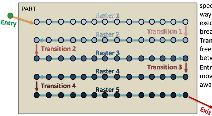
specified Cartesian waypoints to be executed without breaking\* **Transition** - A freespace move between rasters **Entry/Exit** - A freespace move from/to a position away from the part
